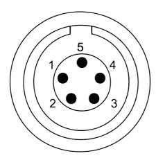
Connection pins (view onto the connector)
