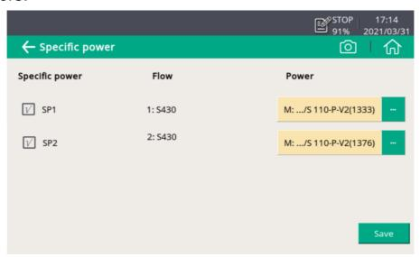
**Specific power** Select to enable the SP channels on the S551 as needed.
