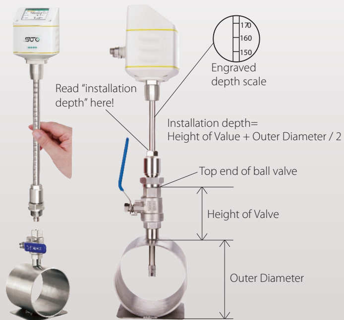
S430 Installation through a ball valve
