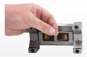
Placing the couplant pads before installation on the transducer surface
